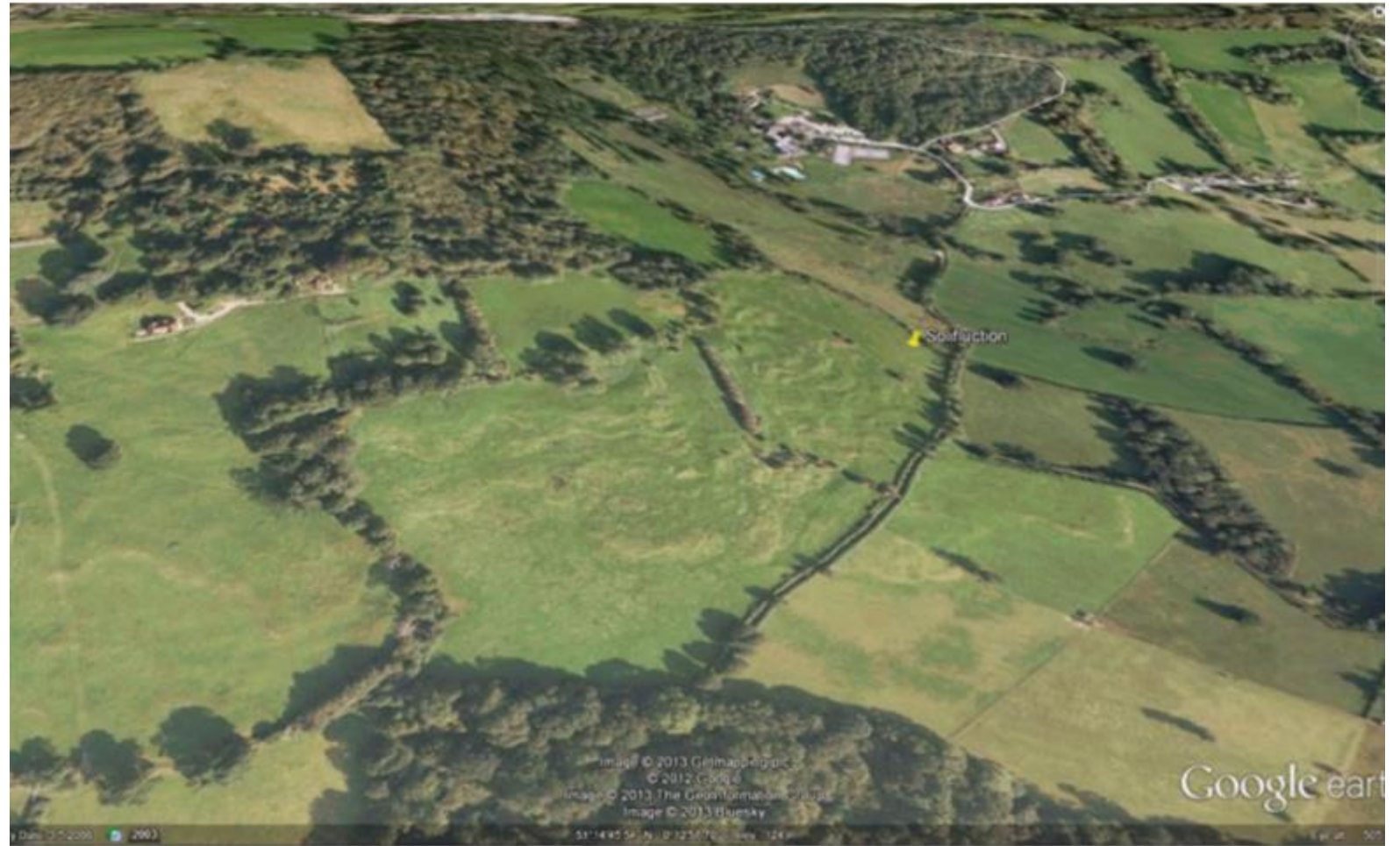
.6. Active-layer detachment slides (previously described as solifluction lobes) in Cretaceous Lower Greensand Formation, adjacent to the Sevenoaks Bypass, Kent. © Google Earth Pro, Getmapping PLC 2012.
