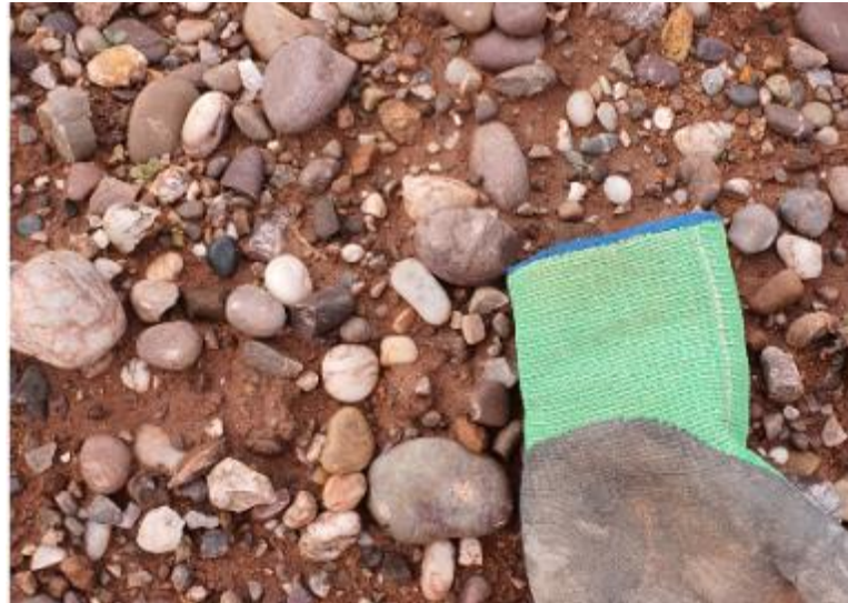
Brown or purple quartzite, with quartz conglomerate and vein quartz. Origin Armorican Massif in France
